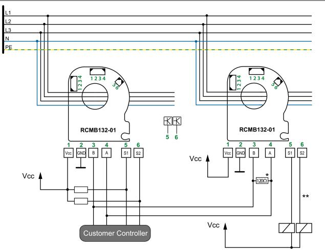
\* Terminating resistor 120  $\Omega$  must only be set on the last device in the RS-485 bus chain \*\* An external protective circuit is especially required for inductive loads.
