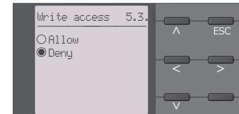
Write access is set to "Deny" when the device is delivered. Parameter changes via the web server are only possible when write access in the device has been allowed.
