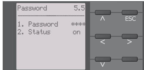
3. Under **Menu/Device settings/Password/Password**, enter a four-digit password using the arrow keys. You can use the numbers 0 to 9.
