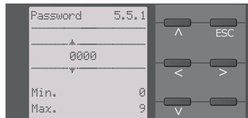
The device is now password protected. Changes in the device are now possible only when the correct password is entered.
